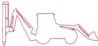
Mounting to a Rubber Tyred Back Hoe - RX100 Option
